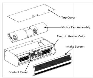
FIG. 1 (Electrically Heated STD2 unit)
