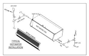
FIG. 3 (Hot Water Heated STD Unit)
