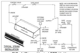
FIG. 4 (Steam Heated STD Unit)
