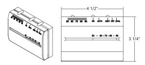
99-264 – Thermostat, 24 Volt, Analog, Single Stage, R.G.W.Y.B.O.
