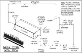
FIG. 4 (Steam Heated STD Unit)
