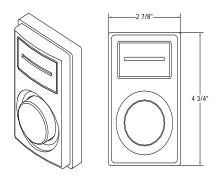
99-063 – Thermostat, 801, Line Voltage, Single Stage, Single Pole
