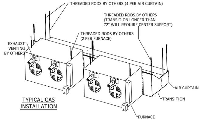
FIG. 5 (Indirect Fired Gas Heated HV Unit)
