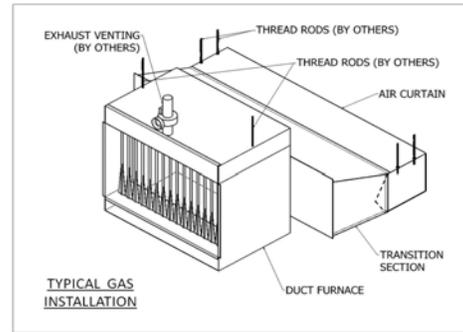
FIG. 5 (Indirect Fired Gas Heated HV Unit)
